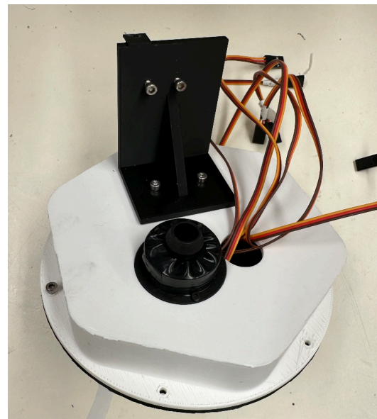
Figure 10: Picture of the assembled housing with base, lid, bracket, pneumatic adaptor, and primary servo motors (inside housing)
